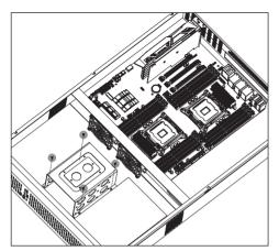
7. Install HDD cages and GPU Holder.
