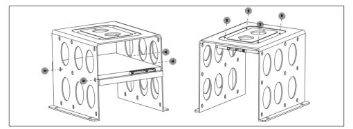
5. 4x 3.5" HDD and 2x 2.5" SSD (or total 6 x 3.5" HDD) can be installed on the HDD cages.
